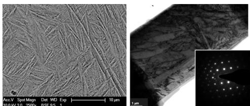
Figure 1: SEM and TEM micrographs of as-built SLM sample. The microstructure is fully martensitic  $\alpha'$  phase.
