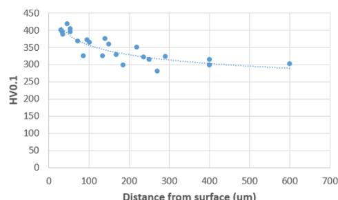
Figure 2: Microhardness variation in the HIP(a) treated sample along the cross-section. The variation is consistent with the presence of brittle alpha case layer rich in oxygen.
