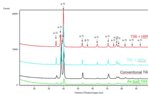
Figure 3: Microstructure and XRD diffractograms after HIP treatment. The main phases detected are  $\alpha$ - and  $\beta$ -Ti.
