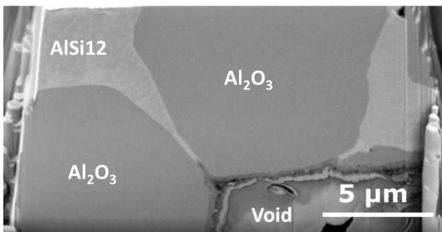
Figure 1: A cross-section view from 3D FIB volume reconstruction of a representative volume of the 3D printed AISi12/  $\text{Al}_2\text{O}_3$  MMC.
