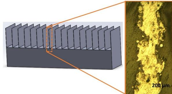
Figure 2: Design of single laser-track walls manufactured and the best quality observed wall with 15vol% of  $\text{Al}_2\text{O}_3$  is shown.
