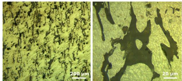
Figure 3: Microstructure of 15vol%  $\text{Al}_2\text{O}_3$  of 3D printed MMC using the so far optimized laser parameters and 50% hatch distance overlap.
