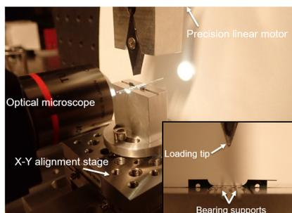
Figure 2: Mesoscale compression test bench in 3-point bending setup.
