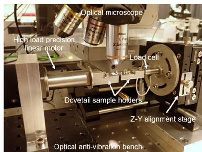
Figure 1: Mesoscale tensile test bench.
