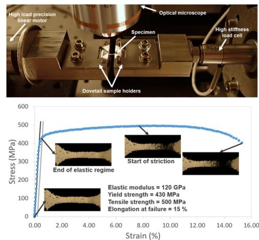
Figure 3: Specimen in the tensile test setup. Images taken during the test using optical microscope are used in DIC to calculate deformations.
