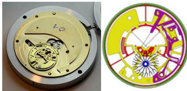
Figure 2: SILOSCAPE escapement (right) integrated in a watch caliber (left).
