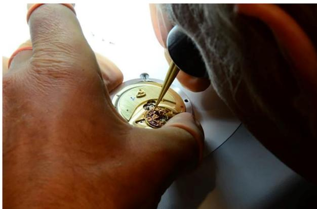
Figure 1: Assembly of the SILOSCAPE escapement in a watch caliber.
