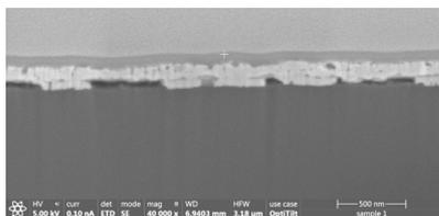
Figure 1: FIB-made cross section of a noisy electrical contact to SiC.
