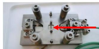
Figure 2: Fixture to apply pressure on SiC chip for LADB hermetic sealing. The arrow shows direction of the hidden thin-wire thermocouple.
