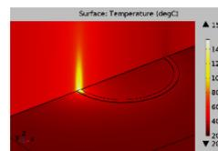
Figure 3: Cross-section of Comsol thermal model (non-calibrated) to show laser induced temperatures on the sealing ring and on the SiC chip.
