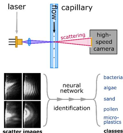
Figure 1: (top) Liquid with suspended particles is run through a narrow capillary. A laser crosses the capillary and produces 2D scattering patterns that are recorded by a high-speed camera. (bottom) The recorded scatter images are analyzed by a neural network to identify the particles, by assigning them to one of the pre-trained classes.
