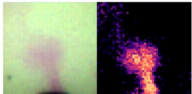
Figure 3: Visualization of  $\text{NH}_3$  vapors coming out from a bottle: left composite image (left), concentration map (right).
