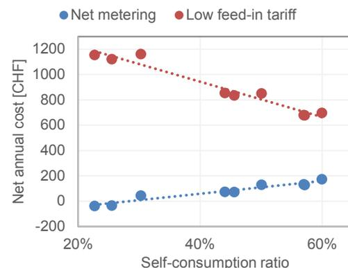
Figure 2: Net annual electricity bill as a function of self-consumption ratio and electricity price configuration. The different SCR values are obtained with different combinations of controllable equipment.
