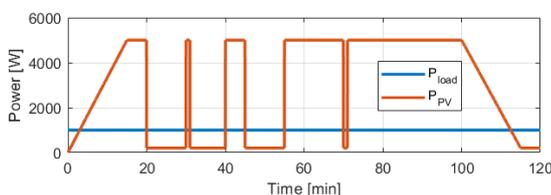
Figure 1: Synthetic test profile to access internal parameters of the EMS. Blue line: house electricity consumption; red line: PV production.
