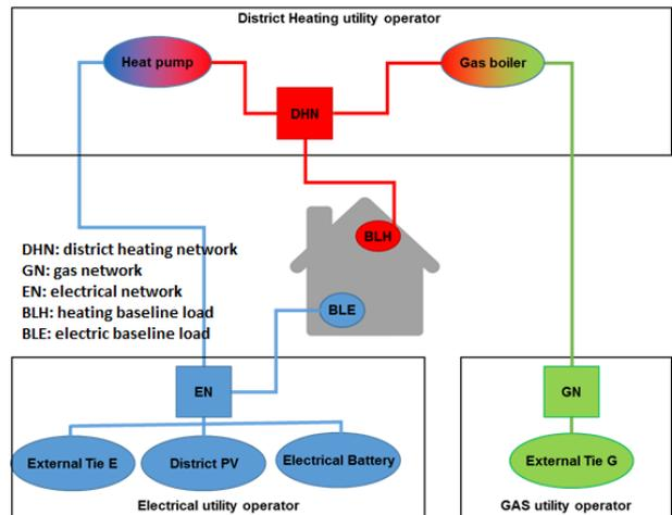
Figure 1: Component diagram of an eco-district with energy carriers interconnected through energy conversion systems (heat pump and gas boiler).
