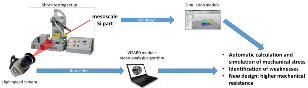
Figure 1: Schematic representation of the proposed system.
