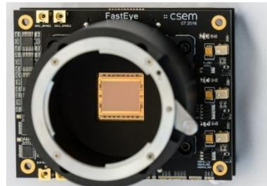
Figure 2. FastEye high-speed camera.
