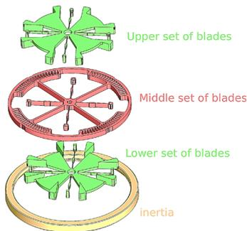
Figure 2: The CR4 mechanical oscillator – exploded view.
