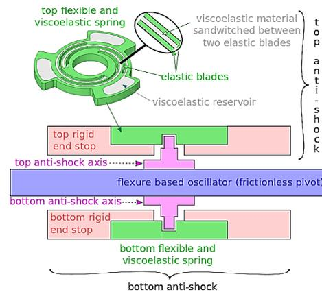
Figure 3: Anti-shock for flexure based mechanical watch oscillators.
