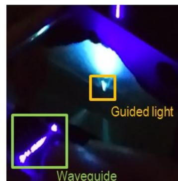
Figure 3: Light barrier printed across a channel to detect air bubbles or particles in the fluid.
