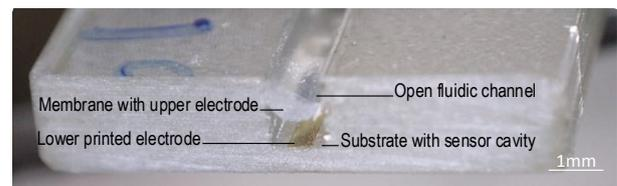
Figure 2: Cross section of a printed pressure sensor flush with the fluidic channel. Covertape to close-off channel not shown.
