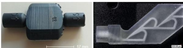
Figure 1: Pump with integrated check valves for mechanical actuation (left); Printed Tesla valve (right).
