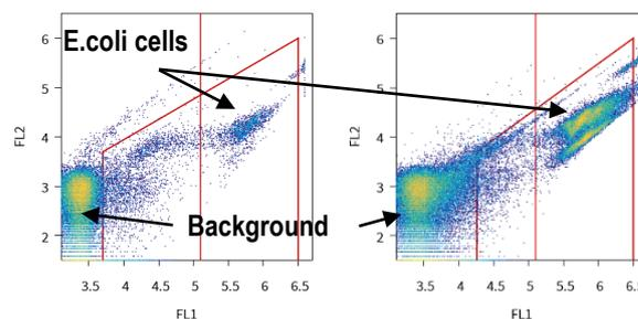
Figure 2: Flow cytometric analysis of a water sample contaminated with *E. coli* cells ( $10^5$  and  $10^6$  CFU/ml).
