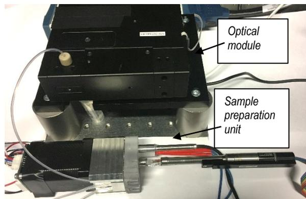
Figure 1: Configuration of miniaturized flow cytometer consisting of a fluidic sample preparation unit, a multi-wavelength optical readout module (scattering and fluorescence) and real-time data processing algorithm.
