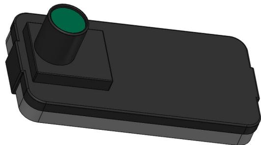
Figure 3: The reading device is developed as an accessory for a 5.2" smartphone with an Android OS. It includes low consumption electronics, battery, proximity sensor, a photodiode, and Bluetooth communication.
