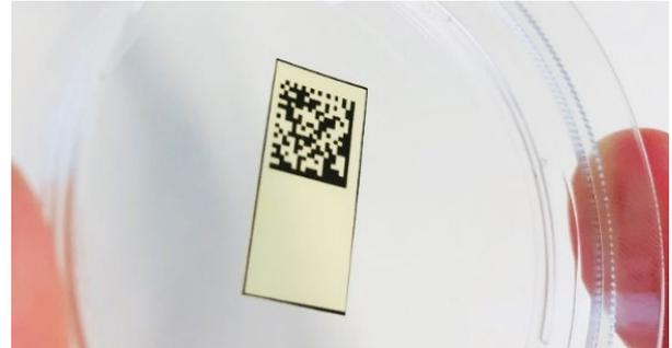
Figure 2: Disposable oxygen sensor (1 x 2 cm) with a printed matrix barcode using a biocompatible ink.
