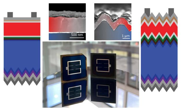
Left and right panels: Schematics of perovskite-on-silicon tandems that are either flat or textured on their front side. Upper central panels: scanning electron microscopy images of the two types of devices developed by EPFL and CSEM. Lower central panels: corresponding picture. Credit: D. Türkay (EPFL), C. Wolff (EPFL), F. Sahli (CSEM), Q. Jeangros (CSEM).
