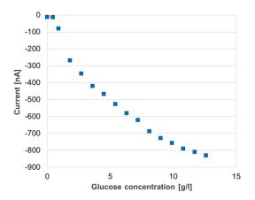
Figure 3: Calibration curve for glucose in buffer solution.
