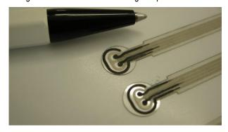
Figure 2: Screen-printed dual electrode sensors for multiple parameter monitoring.
