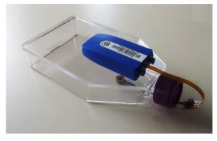
Figure 1: The online cell culture monitoring system CITSens Bio, adapted for the use in a T-flask.
