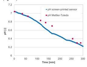
Figure 4: Correlation between the pH measurements in a yeast cell culture performed by a Mettler Toledo pH probe and the C-CIT pH screen-printed sensor.
