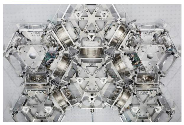
Each of the six hexagonal tiles supports a small mirror and is connected to the others to form a single, larger mirror.
