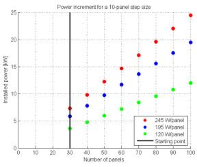
Figure 1 How installed power is incremented (Solar Calculation)
