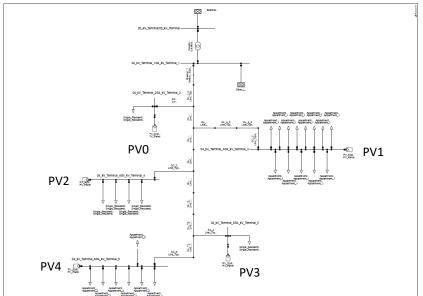
Figure 21 CIGRE benchmark low-voltage microgrid network
