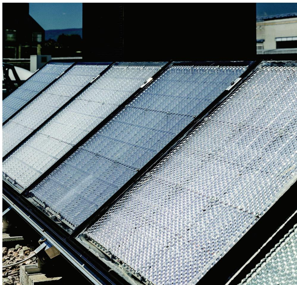
Using an optical micro-tracking process that concentrates sunlight, Insolight's technology achieves 29% efficiency in the pre-production phase. @Insolight
