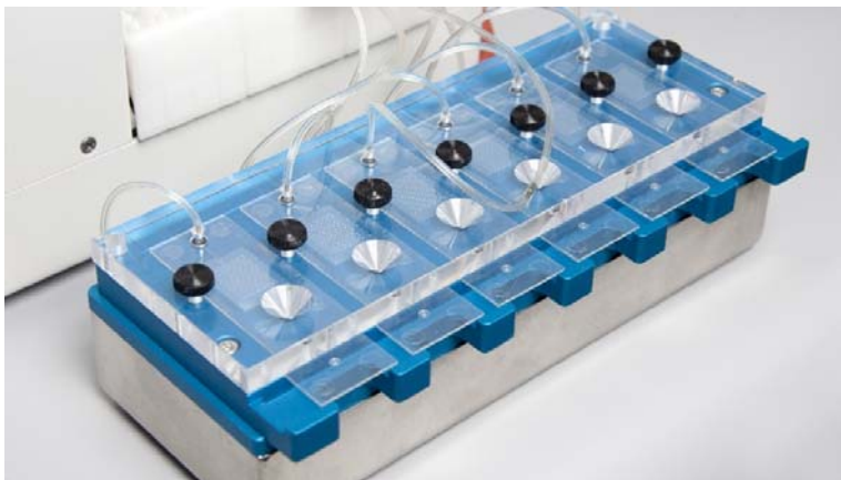
Prototype of the bioanalytical fluidic system. The system allows the simultaneous processing of six biochips for the analysis of six patient samples.
