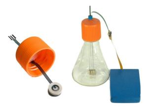
Figure 1: The CITSens Bio online cell culture monitoring system; (left) the sensor is introduced in cell culture systems caps; (right) the sensors in a suspended culture flask, and connected to the wireless data transmission system [1]
