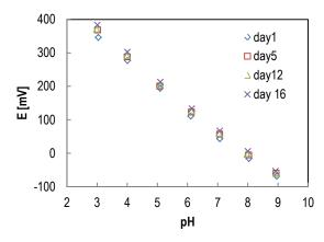
Figure 3: Calibrations for an all-solid-state pH sensor recorded between day1 and day16 of the monitoring of the sensor
