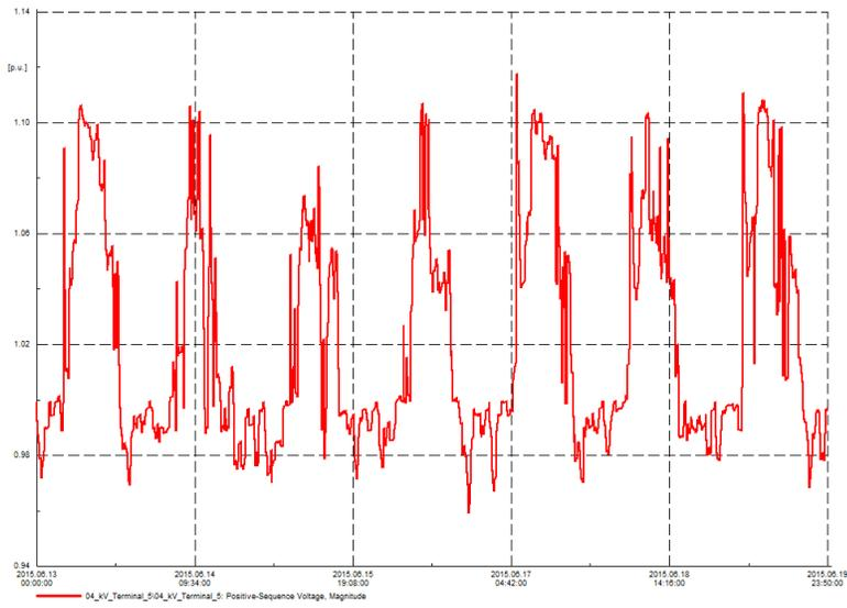
Figure 24 PCC voltage near PV3
