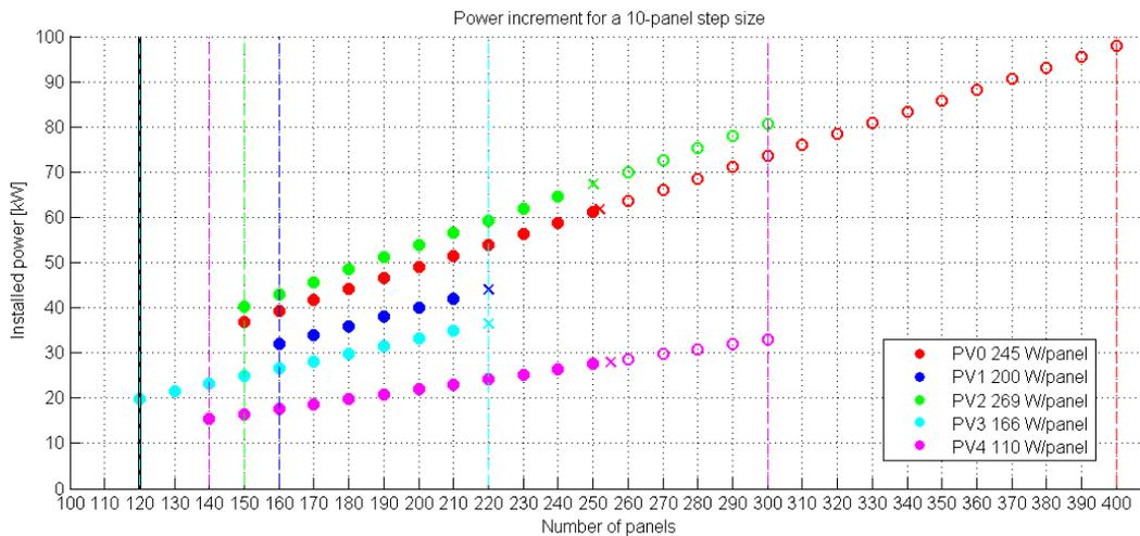
Figure 23 PV hosting capacity results
