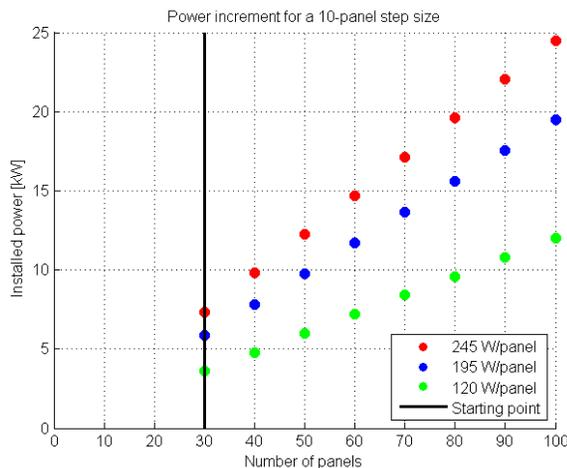
Figure 1 How installed power is incremented (Solar Calculation)
