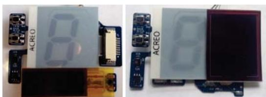
Figure 1: The generic flexible and wireless autonomous platform (left) and generic platform equipped with bigger PV cell for more autonomy.
