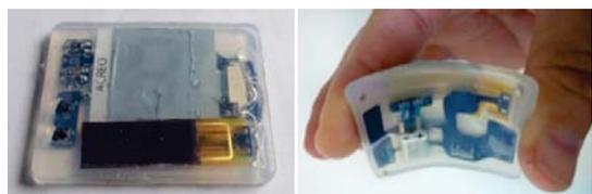
Figure 3: Surrounding coating applied on the flexible patch.
