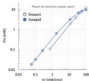
Figure 2: Power available at the maximum power point for the two thin-film silicon PV cells measured under various irradiances.
