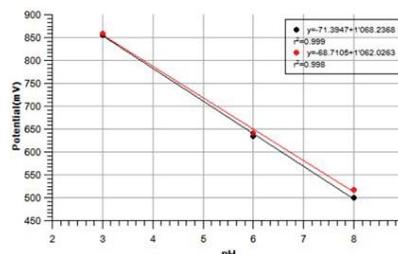
Figure 4: Calibration curve at 3 different pH before and after the sterilization.
