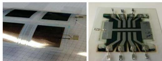
Figure 5: Printed, capacitive pressure sensors as a part of GWAPO platform in hybrid integration approach (left) and printed, flexible solar cells as a part of GWAPO platform in hybrid integration approach (right).
