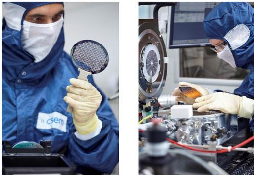
*Manufacturing MEMS atomic vapor cells in CSEM's cleanrooms*
