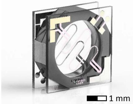
*MEMS atomic vapor cell. Dimensions: 4 x 4 x 1.4 mm.*
