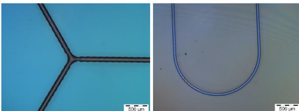
Figure 2: Printed optical waveguide geometries.
