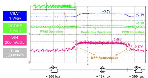
Figure 3: SoC measurement when varying the illumination condition.
