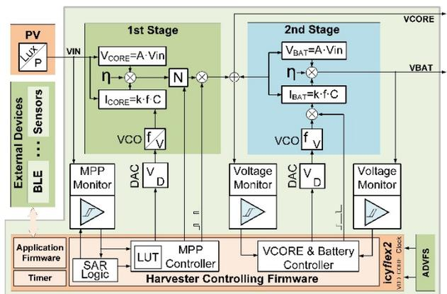
Figure 2: Block diagram of the dual stage energy harvesting unit.
