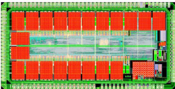
Figure 1: Smart powering unit SoC layout comprising a fully-integrated switched-capacitor based harvester, two MCU cores, 32 KB SRAM, 8 KB ROM, standard peripherals and interfaces.
