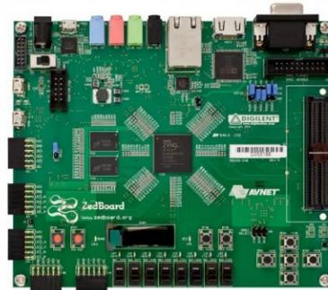
Figure 2: ZedBoard with a Xilinx ZYNQ 7020 FPGA.
