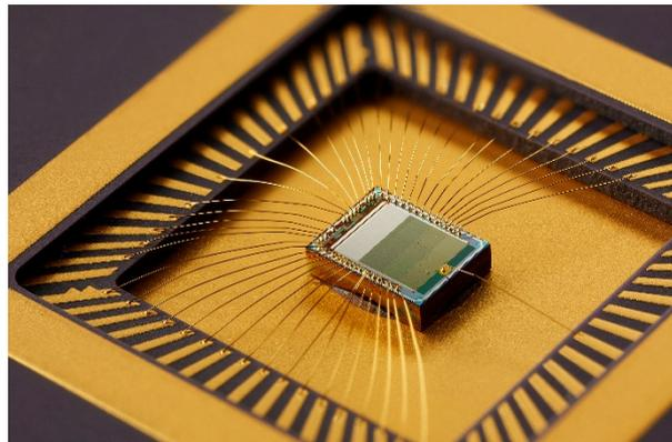
Figure 2: Microphotograph of the chip with top part of the chip unmodified and the lower part (3×3 square array) showing the amorphous photodiodes with 100% fill factor.
