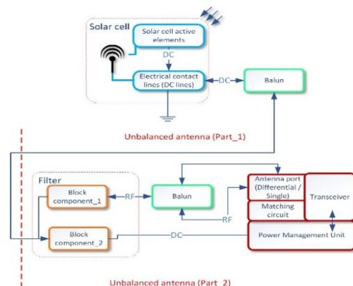
Figure 2: Block diagram of the proposed antenna system solution.
