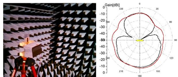
Figure 3: Antenna under test: radiation pattern measurements (CSEM anechoic chamber).
