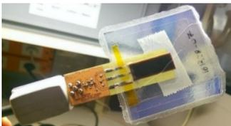
Figure 1: Solar cell element antenna prototype.
