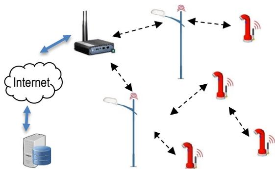
Figure 1: Lorno wireless water distribution network monitoring system.
