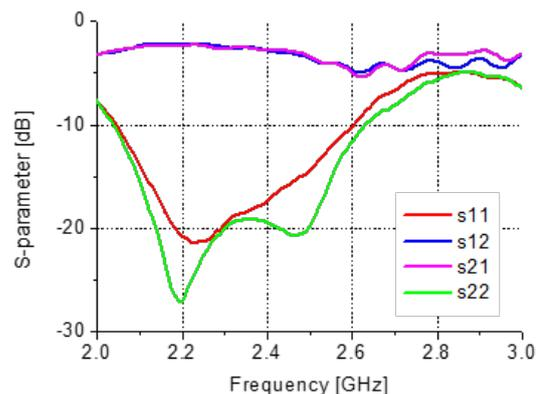
Figure 2: Sample of the waveguide under test (top) and its measured performance characteristics (bottom).
