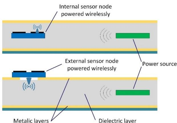
Figure 1: General concept of a sensor node remotely powered via RF energy harvested from a RF source and distributed via the FWG.
