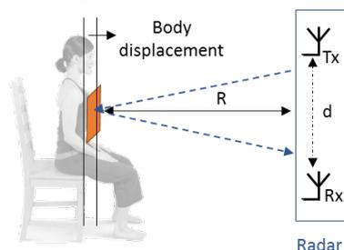
Figure 1: Radar-based VS measurement principle.
