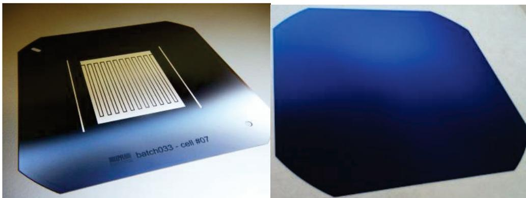
Back-side view of the solar cells (here on a larger wafers) with positive and negative contact.
