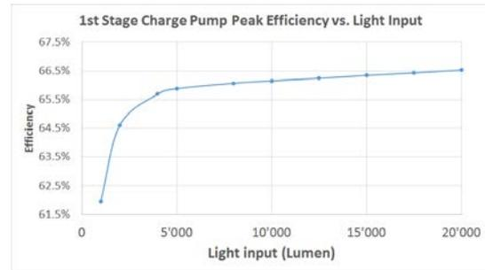
Figure 2: The simulated peak efficiency of the 1st stage as a function of illumination.
