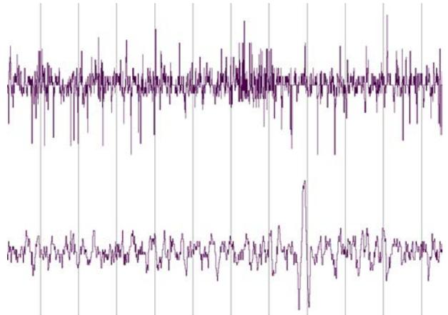
Figure 2: Simulation results of the correlation peaks obtained in the receiver: the first plot is the input signal, the second is the access address correlator output. The correlation peak is clearly visible.
