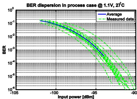
Figure 1: BER sensitivity at 2 Mbps measured over several samples.
