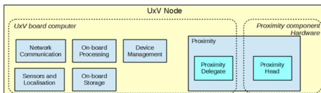
Figure 1: the RAWFIE UxV Node architecture including the Proximity component.
