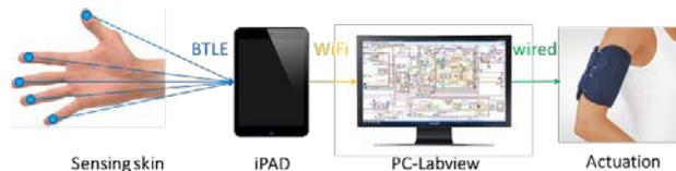
Figure 3: WiseSkin prototype 1 test configuration.
