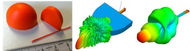
Figure 2: Prototyped 3D plastic antennas (left) and corresponding HFSS computational models with theoretical radiation patterns (right).
