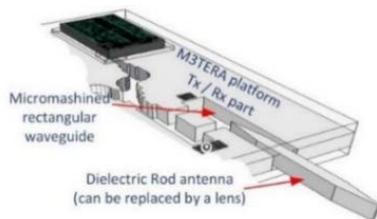
Figure 1: General drawing of the M3TERA miniature platform module.
