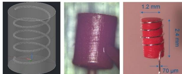
Figure 3: Helix antenna (from left to right): antenna model, realized 3D solution with helix inside and helix wire outside (TeraExplore project).
