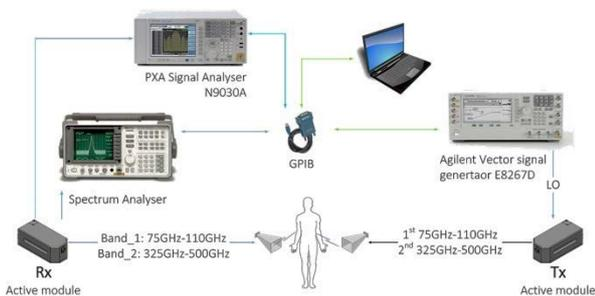
Figure 1: Measurement setup.
