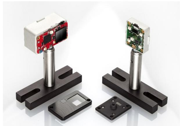
Figure 2: Sensor (left) and tracker (right) prototypes mounted on optical posts (front covers removed).
