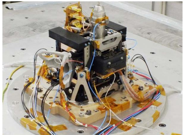
Figure 2: EQM instrumented and mounted on vibration shaker table.
