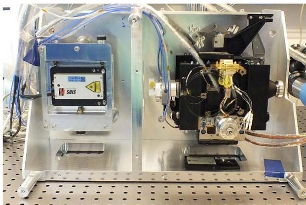
Figure 1: EQM mounted on performance test bench with interferometer in ISO5 (Class 100) cleanroom conditions.
