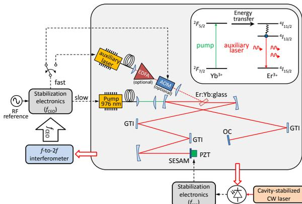
Figure 1: Schematics of the femtosecond DPSSL architecture with the external modulation laser source acting on the laser Er<sup>3+</sup> transition of the Er:Yb:glass gain medium for stabilization of  $f_{CEO}$ .  $\lambda_{emission} = 1554$  nm,  $f_{rep} = 100.05$  MHz, pulse duration: 165 fs (transform-limited). (Inset) Energy diagram of the Er:Yb:glass system with stimulated emission modulation of the gain from the auxiliary laser.
