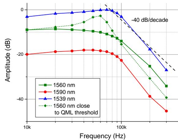
Figure 2: Transfer function of the auxiliary laser power to femtosecond laser output power with 100% modulation depth, rescaled. For 1560 nm, the transfer function (arbitrarily offset) close to the QML threshold shows a typical oscillation relaxation resonance at about 57 kHz.
