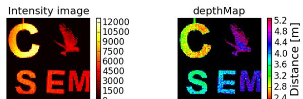
Figure 4: Images generated by the LiDAR (intensity on the left and distance on the right).
