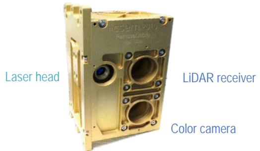
Figure 2: VBN sensor with laser head, LiDAR receiver, and camera.
