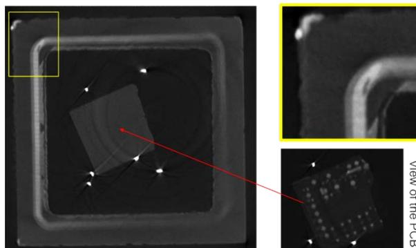
Figure 2: Example of cross-section images obtained with the high-resolution XPCI system. Defects can be observed in the bonding line (yellow-framed inset).
