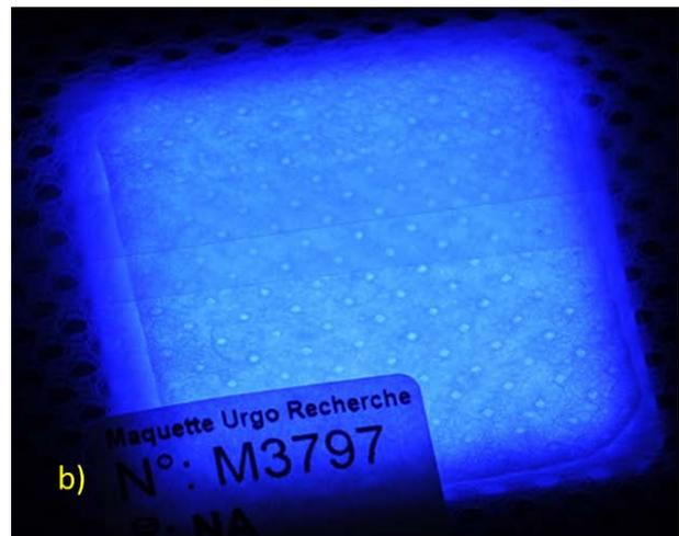
Figure 2: First demo of the thin 16 cm<sup>2</sup> MEDILIGHT illumination system. The demo consists of 32 LEDs, diverse light management elements for light redirecting and homogenization as well as the complete wound dressing from the industrial partner URGO on top. The illumination system is able to provide high intensities up to 25 mW/cm<sup>2</sup>.
