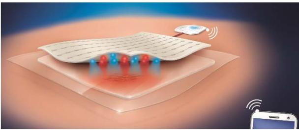
Figure 1: Illustration of the MEDILIGHT wound healing system. It consists of a disposable wound dressing, an exterior flexible illumination system with sensors and the controlling electronics.
