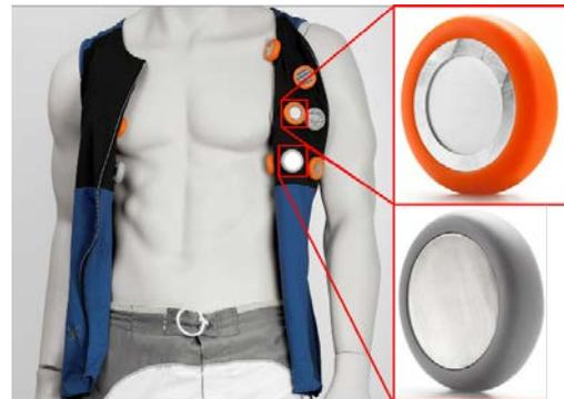
Figure 1: The WELCOME sensor vest (here shown half open) is equipped with 21 sensors (diameter: 38 mm; height: 10 mm), which are in direct contact with the skin and measure a wide spectrum of body signals with a high spatial and temporal resolution.
