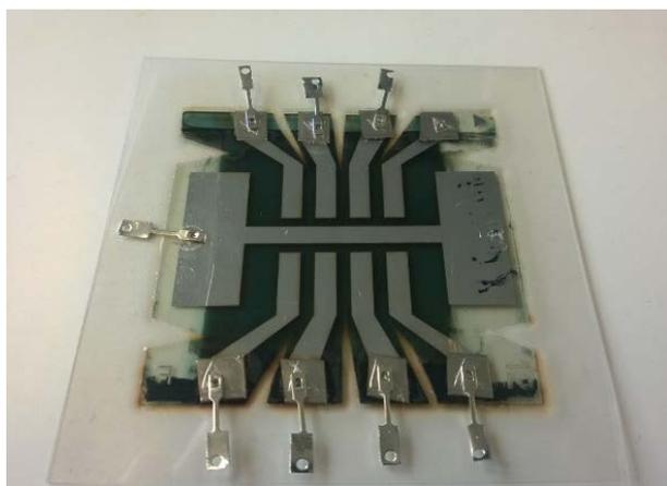
Figure 1: Photograph of the encapsulated flexible tandem solar cells.
