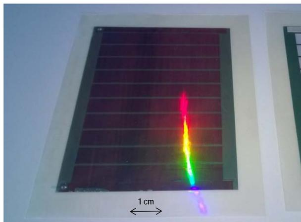
Figure 2: Photograph of one of the final flexible tandem demonstrator modules, encapsulated and laminated with a light management foil.
