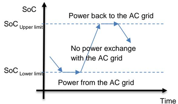
Figure 2: Control strategy of the interface converter.
