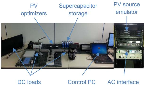
Figure 1: DC micro-grid demonstrator.
