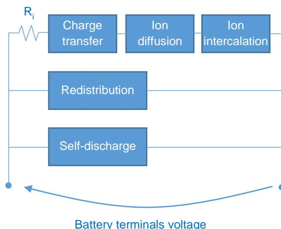
Figure 3: Structure of the dynamic battery model by CSEM.
