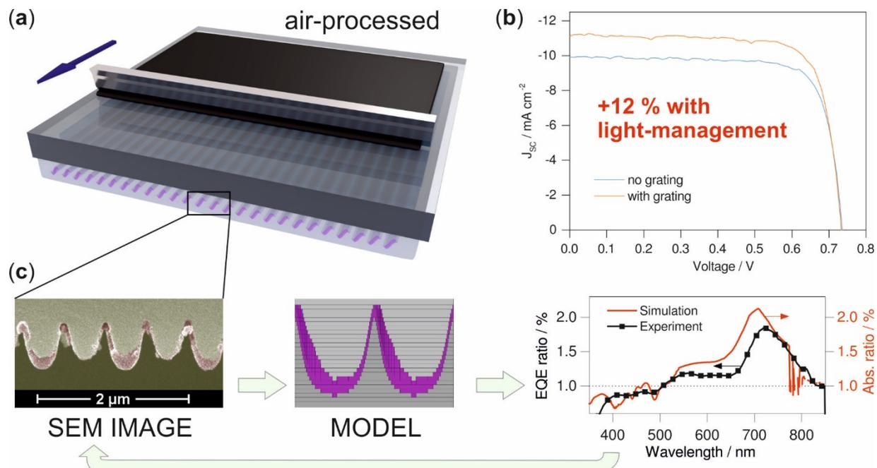
Figure 1: (a) Photovoltaic test cells are printed on a modified substrate with an attached light-management layer. Through light redirection via elaborated diffraction properties, the absorption in the absorber is enhanced and (b) a 12% increase in the efficiency is obtained. (c) A simulation platform was developed to predict, explain and design the impact of the photonic nanostructures for a given cell architecture and use case.
